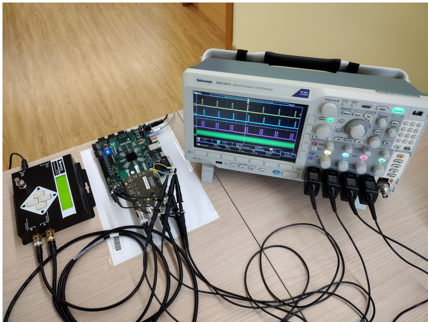
Figure 7: Bench setup showing FMC-SDI card connected to the Digilent ZedBoard and the scope connected to the PMOD header for debug
