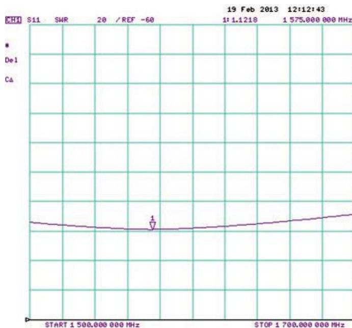
Antenna VSWR on Test Board
