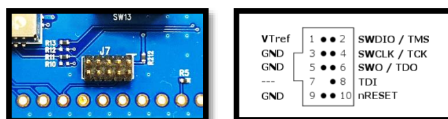
Figure 2: JTAG Pin Connection
