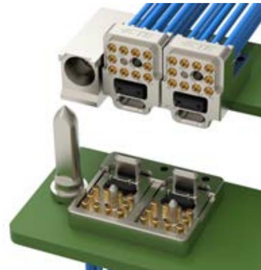
Next Generation VPX module market trends are calling for increased density and bandwidth within an embedded computing slot (more speed and functionality), TE Connectivity (TE) NanoRF hybrid modules leverage a floating Insert in the backplane with guide features that pre-align contacts before engaging reducing potential for damage. These modules offer high density RF and optical connections within a common connector module for VPX-based embedded computing systems.
