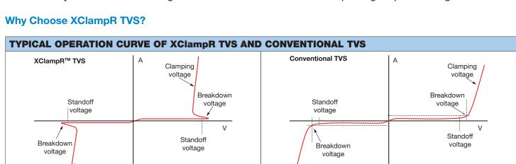
XClampR TVS is a snapback type TVS with an extremely low clamping voltage ratio for suppressing transient voltage to a lower clamping voltage, compared to conventional TVS.
