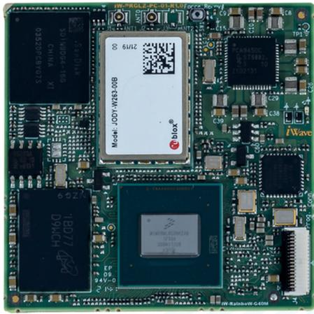
The i.MX 8M Plus SoC based LGA Module is designed as per The Open Standard Module™ specification (OSM).It integrates NXP's i.MX 8M Plus offerings Quad/ QuadLite /Dual Cortex A53 @ up to 1.8GHz, NPU with up to 2.3 TOP/s, HDR capable Image Signal Processor (ISP) with IEEE 802.11 a/b/g/n/ac/ax\* Wi Fi & BT 5.0 module.
