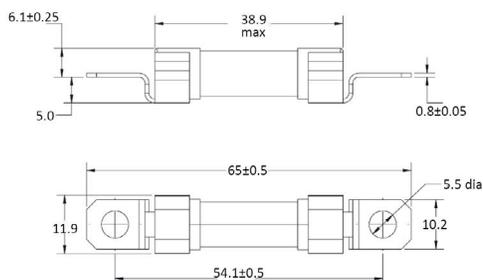
Note: recommend tightening torque is 4.5 ±1.0 Nm for M5 Screw
