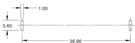
**PCB layout 2P: 2 pin PCB terminal**
