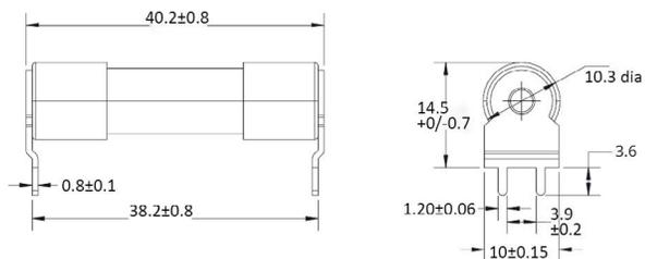
**PCB layout 1P: 1 pin PCB terminal**
