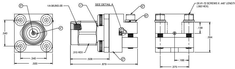
**Low Profile Connectors – (at 0.375" Height)****Jack, Screw-on Type, Low profile, 0.005" Pin**
