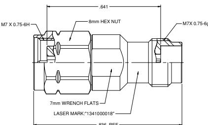
**Adapter Assembly, 1.85mm Plug to 2.4mm Plug**
