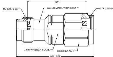
**Adapter Assembly, 1.85mm Plug to 2.4mm Jack**
