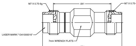
**Adapter Assembly, 1.85mm Jack to 2.4mm Plug**
