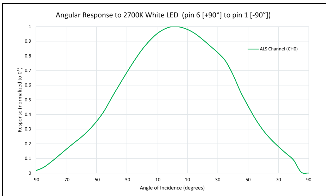
Figure 11: ALS Average Angular Response to 2700K White LED (pin 6 [+90°] to pin 1 [-90°])
