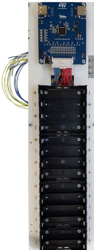
Figure 4. Cables to connect external NTCs
