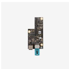
To capture the ZED X on the NVIDIA Jetson AGX platform, one solution is to utilize a GMSL2 capture card that directly connects to the Jetson's CSI port.
