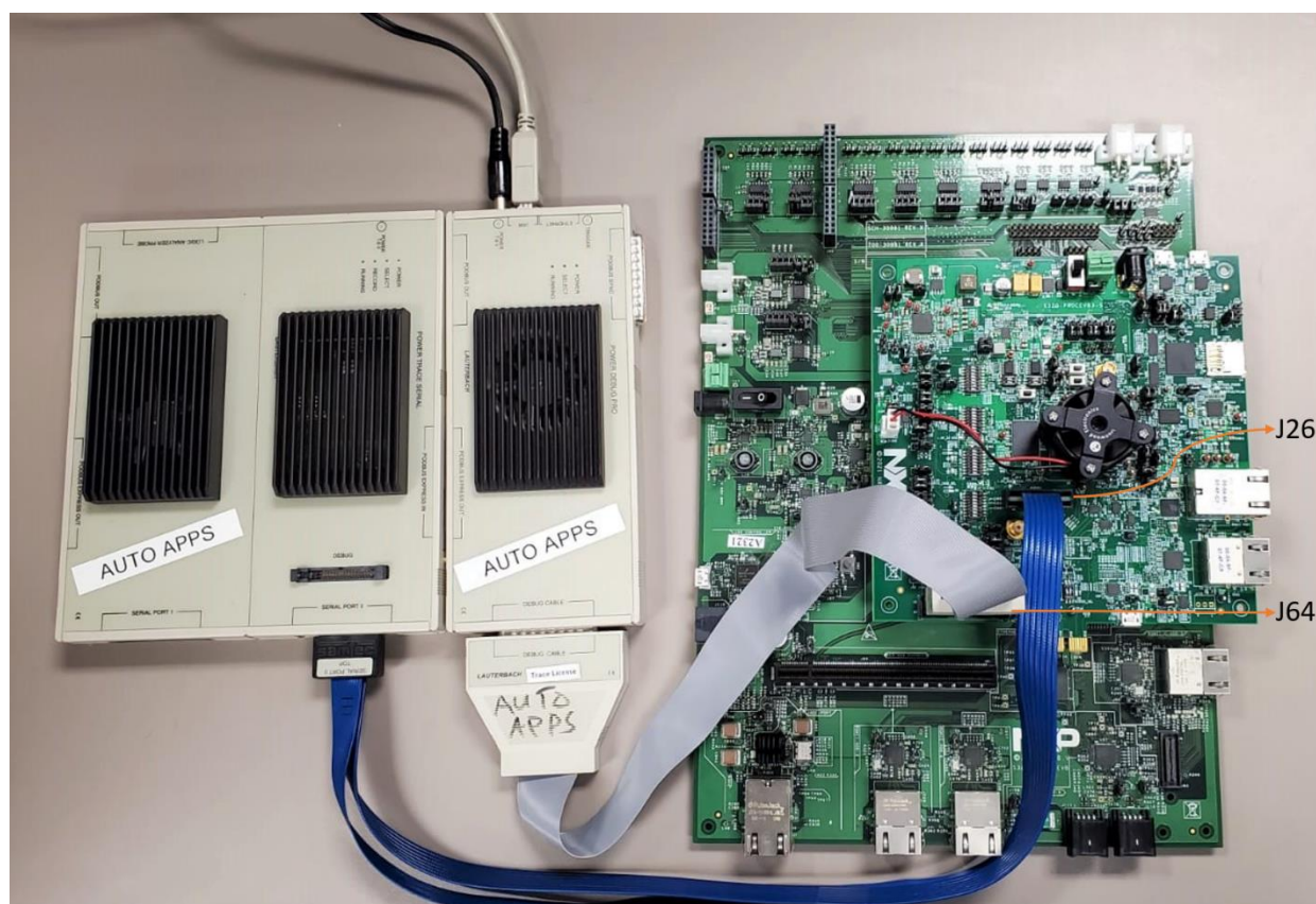
Figure 13. Aurora Port setup 1 with ATP and JTAG cable connected on S32G-VNP-EVB3
