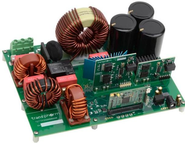
Figure 1. TDTP2500B066B 2.5kW totem-pole PFC evaluation board
