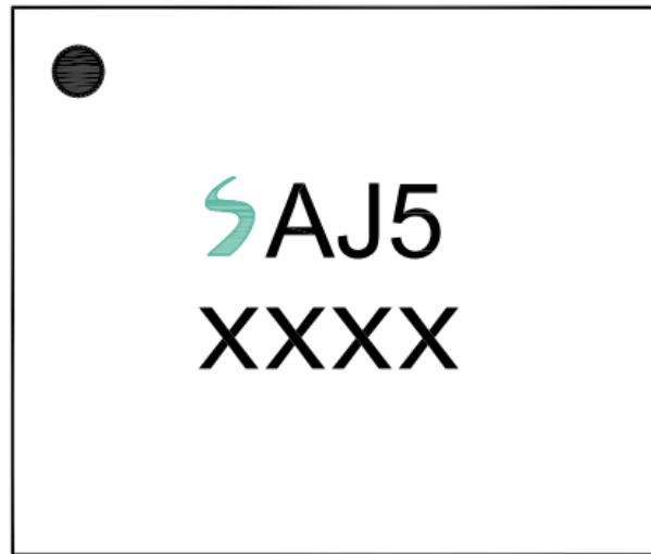
Figure 3: Marking Information – DFN Package
