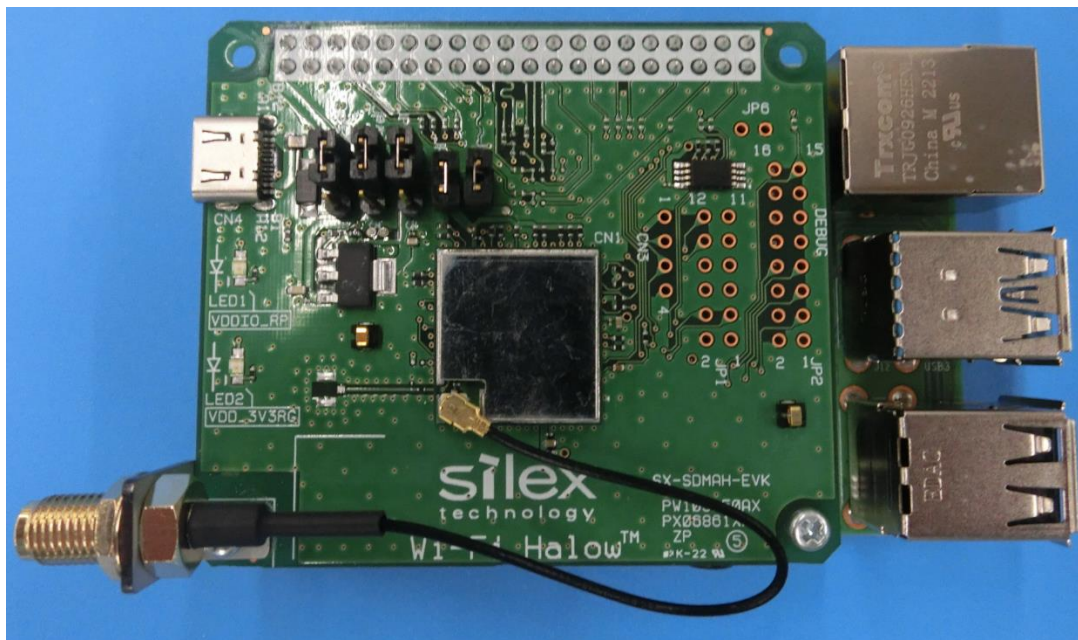
Figure 2: SX-SDMAH mounted on a Raspberry Pi 4
