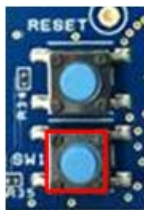
Figure 17. User Switch on EK-RA4W1 Board
