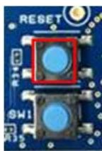
Figure 16. Reset Switch on EK-RA4W1 Board
