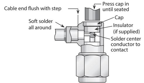
2) Soft solder cable jacket to body, making sure that end of cable is flush with step in body. Solder center conductor into contact slot, assemble insulator disc (if supplied), then press cap into body until seated or screw into place.
