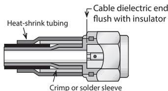
3) Insert cable/contact into rear of body, with all braid wires on outside of crimp tail. Push cable in until cable dielectric bottoms in connector. Trim excess braid wires even with shoulder of body. Slide crimp sleeve forward until flush with body and crimp (see page 211 for hex die sizes). (For solder-type connectors, solder braid to body and sleeve through hole in sleeve.) Slide heat-shrink tubing into place and shrink with hot-air gun.
