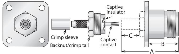
Figure 2 (Contact and insulator captive in backnut)
