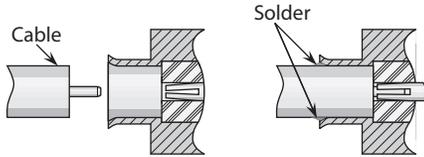
Delta "One-Step" connectors feature captivated contacts and insulators to allow rapid, easy assembly to semi-rigid cable—simply trim the cable jacket and dielectric flush, chamfer the center conductor, insert into the connector, and solder the jacket to the connector body.
