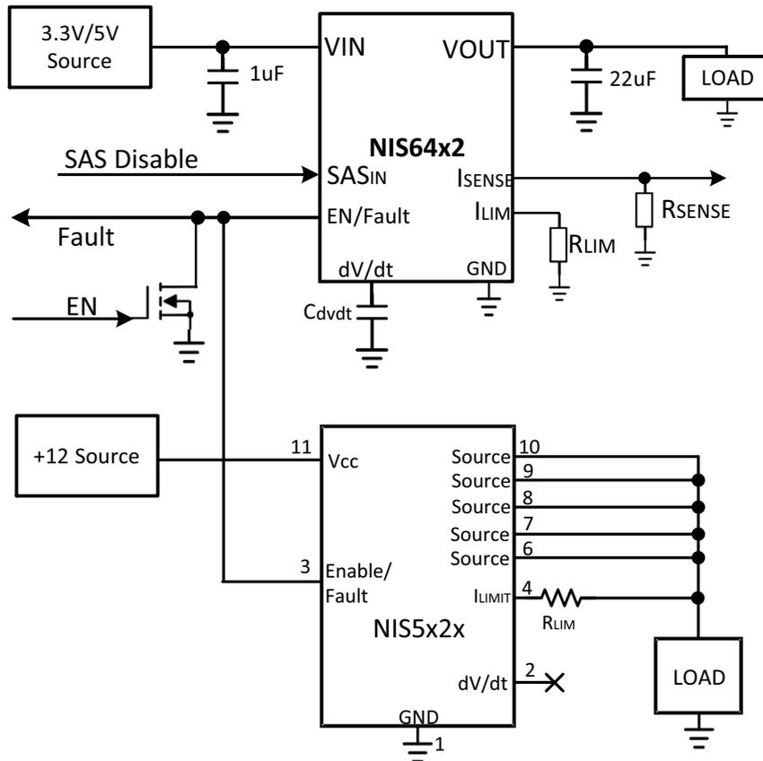
Figure 2. Common Thermal Shutdown with another eFuse
