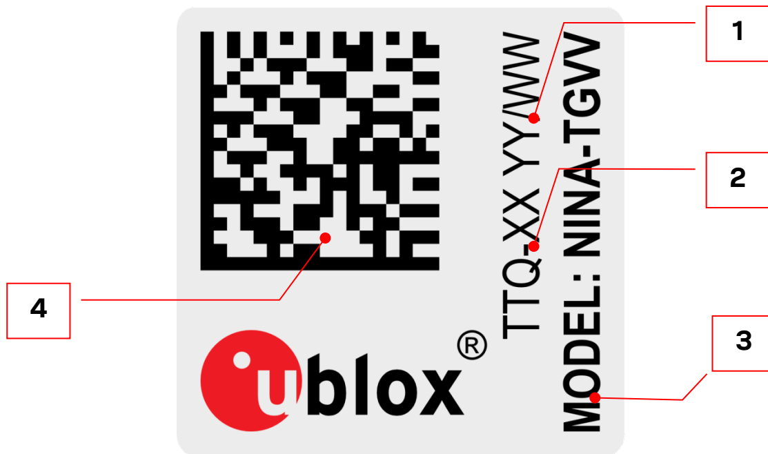
Figure 13: Location of product type number on the NINA-B40 series module label
