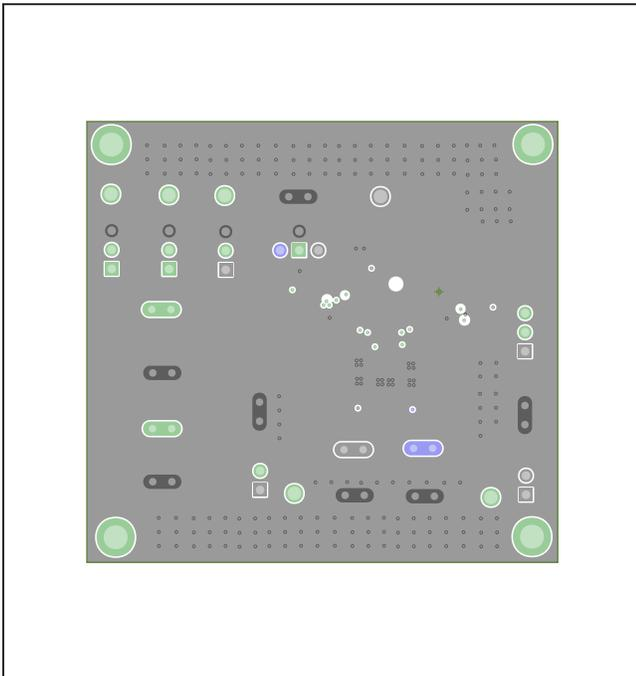
MAX20457 EV Kit PCB Layout - Internal Layer 2
