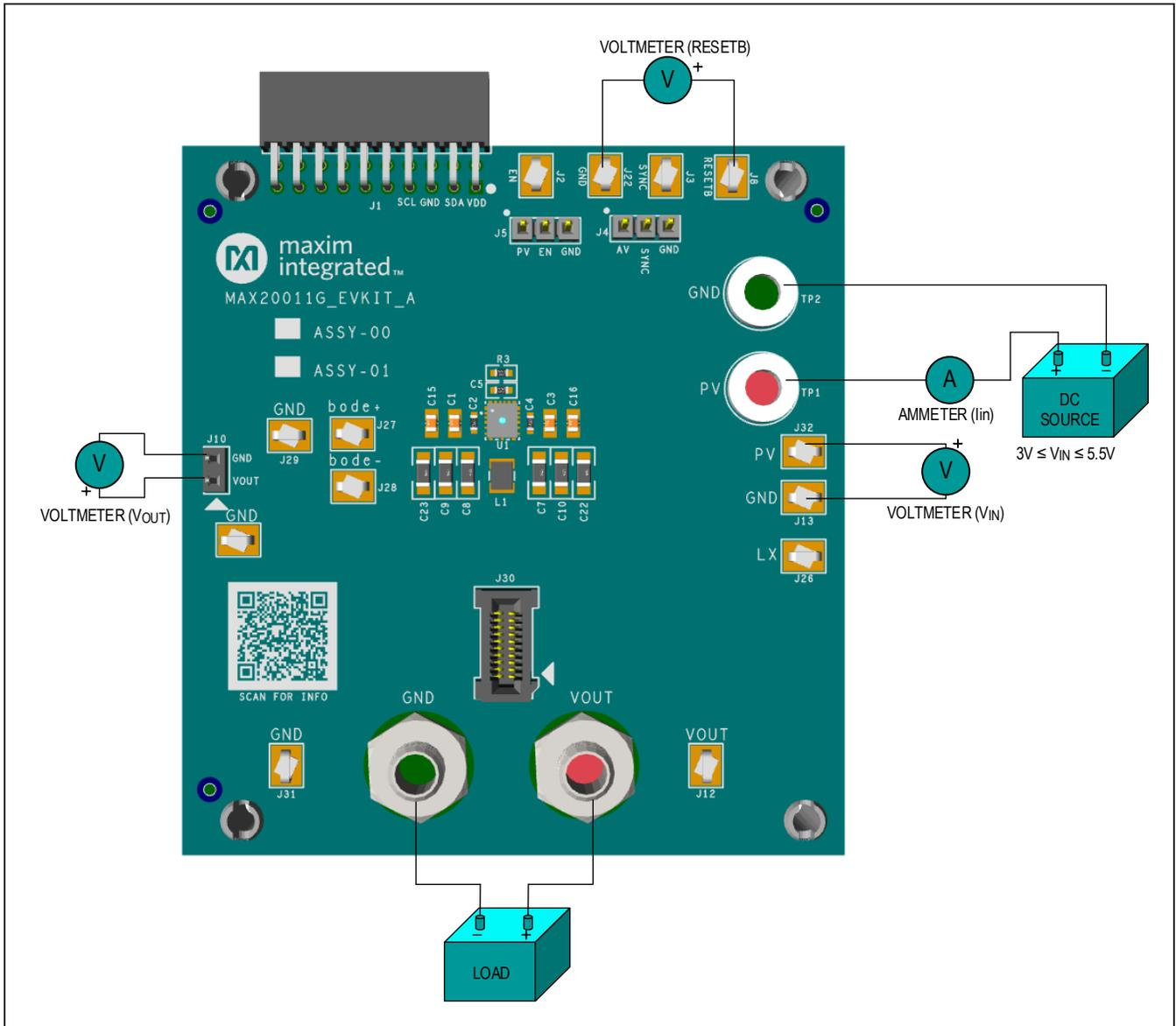
Figure 1. MAX20011G Evaluation Kit Configuration
