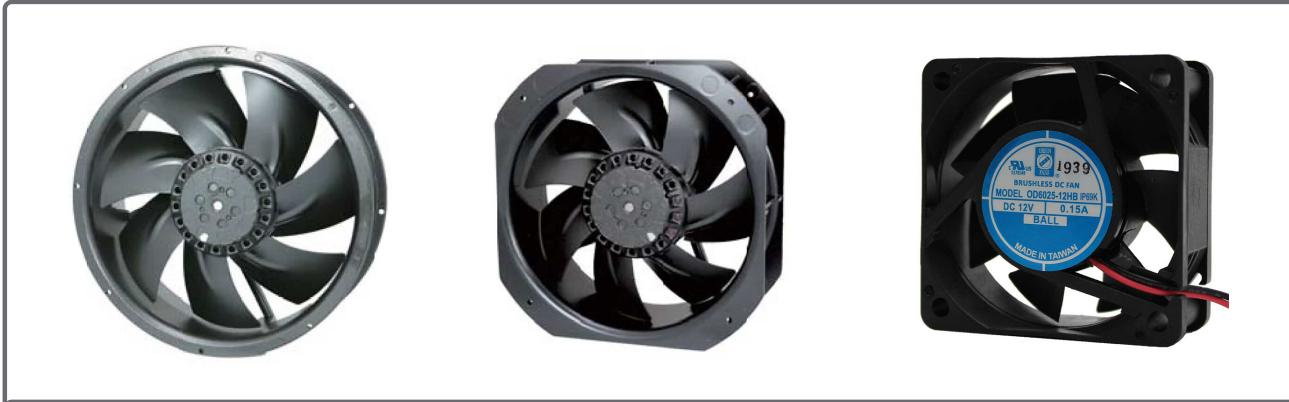
Orion Fans IP69K-rated AC and DC fans are the optimal solution for restrictive environments. The IP69K rating ensures that no damage will occur to electronics during washdown procedures and that no contaminants will enter the fan motor. These fans are rigorously spray tested with 80°C water every 30 seconds with the spray nozzle being 4-6 inches from the fan. The water sprays from 4 angles and is considered a high-pressure stream.
