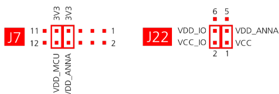
Figure 8: Jumper positions for default power configuration
