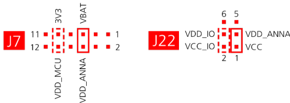
Figure 9: Jumper positions for battery powered operation, two jumpers are optional
