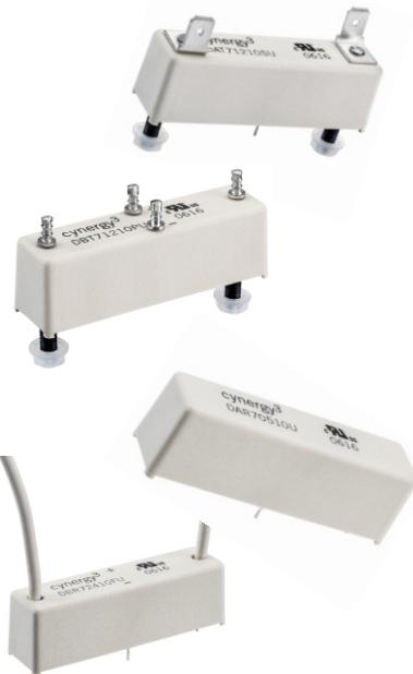
Recently approved by UL, very high isolation voltages (up to 10kV) are achieved through the use of high vacuum reed switches with either Rhodium or Tungsten contacts and make these relays suitable for high reliability applications, such as cardiac defibrillators, test equipment and high voltage power supplies.
