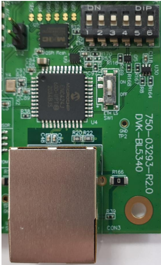
Figure 20: SPI device Ethernet chip (U4), level shifters (U30, Q5, U9), closed DIP switch (S5) schematic and PCB
