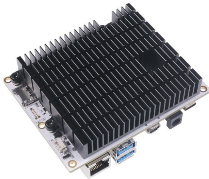
Figure 28. BeagleBone AI-64 back with heatsink at 45° angle
