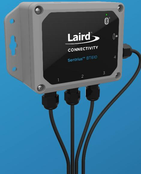
Laird Connectivity's **Sentrius™ BT610 I/O Sensor** with Bluetooth 5 turns your wired sensors into IP67-rated battery-operated wireless nodes, providing robust, secure, and cloud ready messaging. Leveraging our BL654 module, it provides full Bluetooth 5 capabilities, opening up industrial and equipment monitoring applications.
