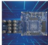
Apollo S10 SoM takes advantage of the latest Intel® Stratix® 10 SoC with 2800K logic elements to obtain speed and power breakthrough (with up to 70% lower power). Combining a number of high-end hardware interfaces such as high-capacity and high-bandwidth DDR4 SDRAM (up to 64GB), on-board USB-Blaster II, and FMC/FMC+ connectors for I/O expansion, the board delivers more than 2X the performance of previous generation development kits.
