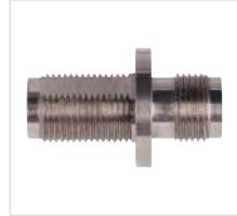
**After 720 Hours of Salt Spray Exposure:**
