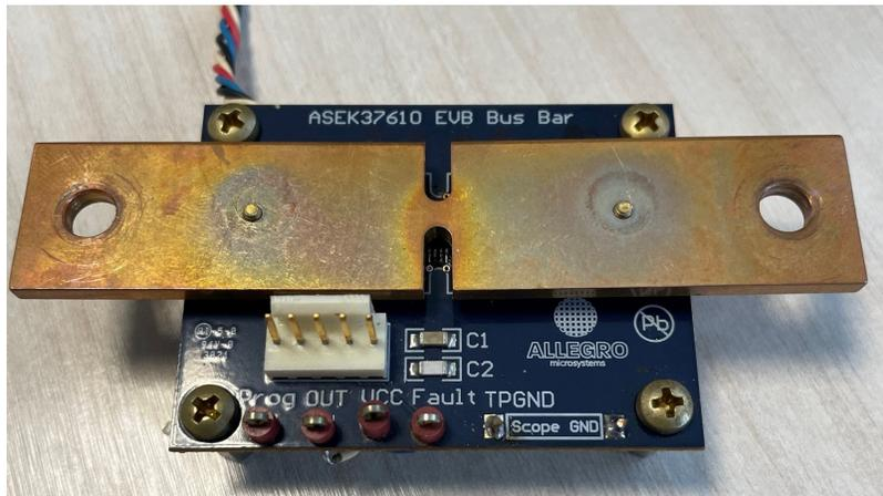
Figure 3: ASEK37610 Test Point Connections
