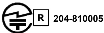
Figure 6: Giteki mark, R and the ANNA-B112 MIC certification number
