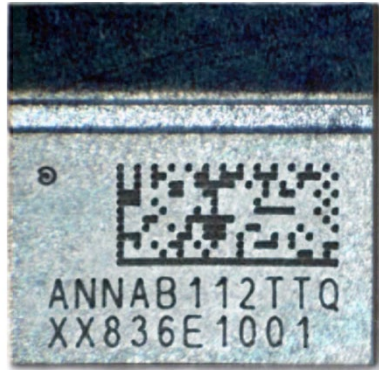
Figure 10: Product marking on the ANNA-B112 module
