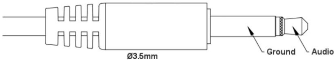
The audio output (headphone) socket is wired: Tip = left, Ring = right, Sleeve = ground
