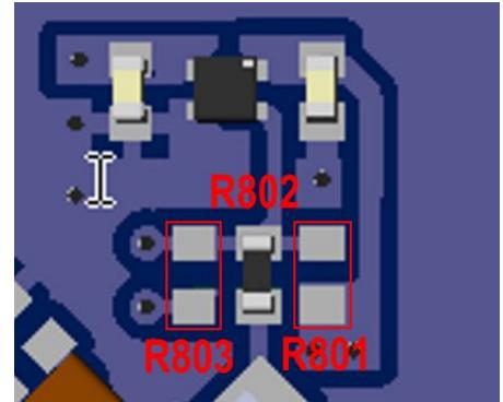
One option to use this feature would be to move R802 to R803, and then install an 0402 100 kΩ resistor at R801. It is not recommended to keep both R802 and R803 installed. Consult the schematic before making adjustments and proceed at your own risk!
