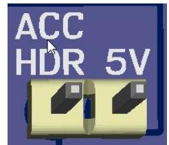
To enable the 5V supply at the edge headers, move the jumper across both pins to join them together. Certain accessory boards require a 5V supply, such as the USB accessory part-number 64006-ES(b).
