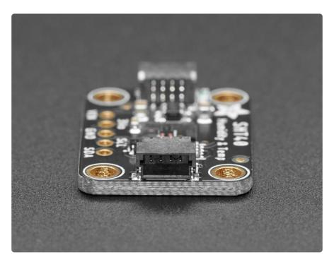
Such a lovely chip - so we spun up a breakout board with the SHT4x and some supporting circuitry such as pullup resistors and capacitors. To make things even easier, we've included <a href="SparkFun Qwiic">SparkFun Qwiic</a> (https://adafru.it/Fpw) compatible <a href="STEMMA QT">STEMMA QT</a> (https://adafru.it/Ft4) connectors for the I2C bus so you don't even need to solder! <a href="QT">QT</a> Cable is not included, but we have a variety in the shop (https://adafru.it/JnB).
