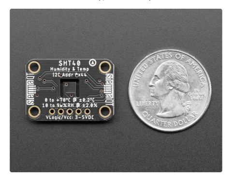
Unlike some earlier SHT sensors, this sensor has a true I2C interface for easy interfacing with only two wires (plus power and ground!). Thanks to the voltage
