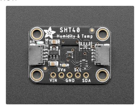
Sensirion Temperature/Humidity sensors are some of the finest & highest-accuracy devices you can get. And finally, we have some that have a true I2C interface for easy reading. The SHT40 sensor is the fourth generation (started at the SHT10 and worked its way up to the top!). The SHT40 has an excellent  $\pm 1.8\%$  typical relative humidity accuracy from 25 to 75% and  $\pm 0.2$  °C typical accuracy from 0 to 75 °C.
