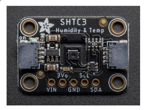
Sensirion Temperature/Humidity sensors are some of the finest & highest-accuracy devices you can get. And with a true I2C interface, reading the data is for easy. The **SHTC3** sensor has an excellent  $\pm 2\%$  relative humidity and  $\pm 0.2$ °C accuracy for most uses.
