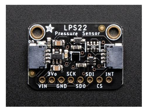
The LPS25 has a wide measurement range of 260-1260 hPa with 24-bit pressure data measurements that can be read up to 25 times a second (Hz), you can be confident that you always have an up to date and precise measurement. The LPS22 has the same measurement range but offers additional measurement rates of 50 and 75Hz. They're pretty dang accurate too, with the ability to measure within 0.2 hPa after calibration (± 1 hPa before calibration).
